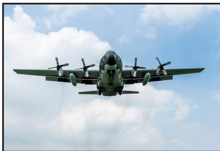
Image: A Taiwan Air Force C-130 transport plane, a four-engine turboprop military transport aircraft made in the United States, about to land at Taipei Songshan Airport, Taiwan. 22
